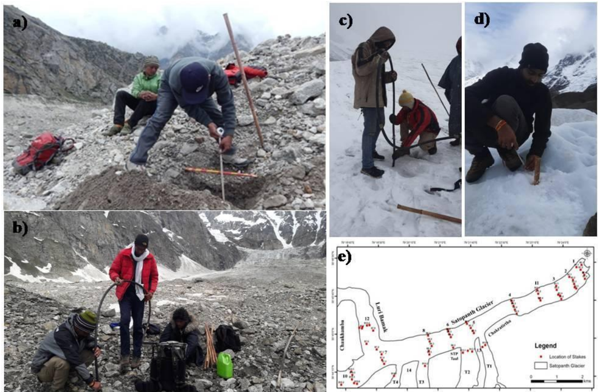
Figure 1. Field photograph showing installation of stakes in debris-covered region (a) in partial debris-covered (b) and clean ice parts (c& d) of Satopanth glacier at an altitude of 3950, 4500 and 4590 m amsl respectively. (d) Network of installed stakes in the year 2019 to assess the glacier health/dynamics.
