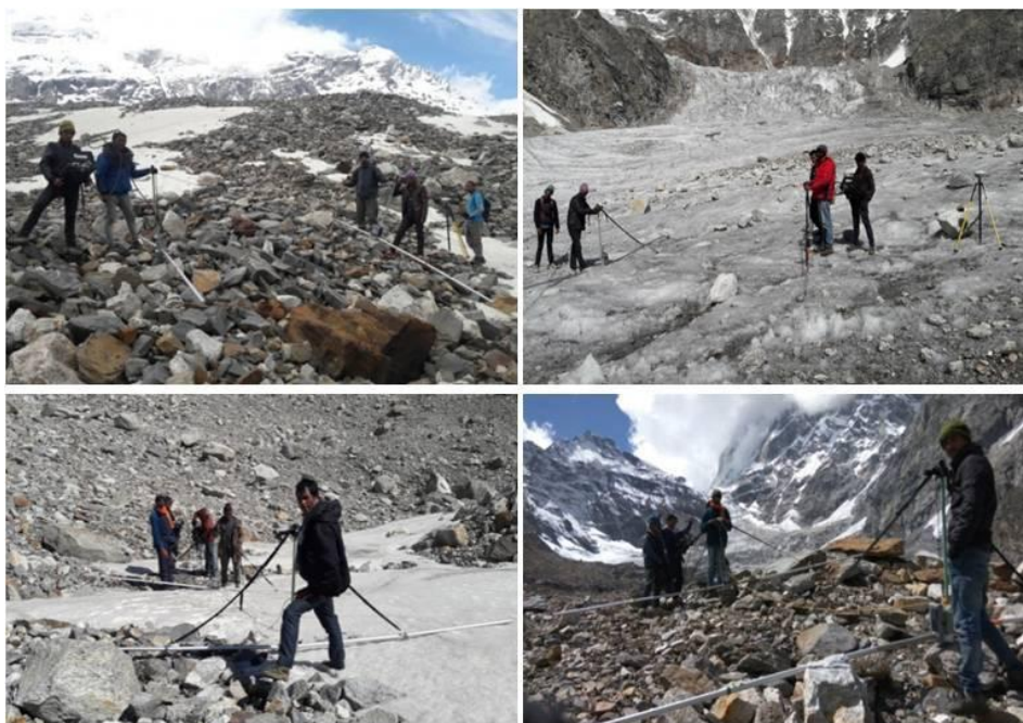
Figure 2. Measurement of ice thickness of Satopanth glacier, Uttarakhand Himalaya using Ground Penetrating Radar.
