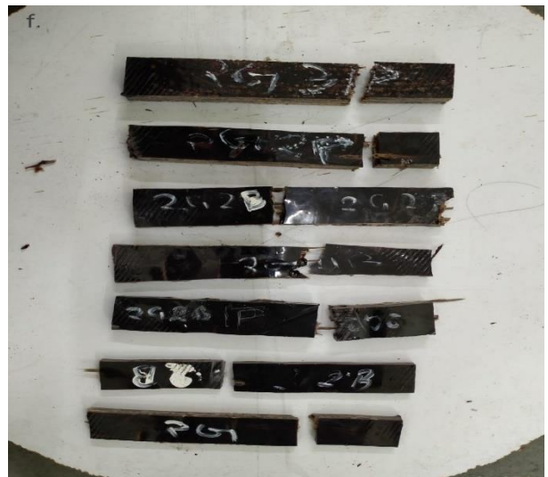
Figure : These figures (a.) , (b.) , (c.) , (d.) , (e.) and (f.) shows the samples after ultimate tensile strength testing of polymer composites samples prepared during the experimentation and project work.
