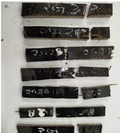
Figure : These figures (a.) , (b.) , (c.) , (d.) , (e.) and (f.) shows the samples after ultimate tensile strength testing of polymer composites samples prepared during the experimentation and project work.
